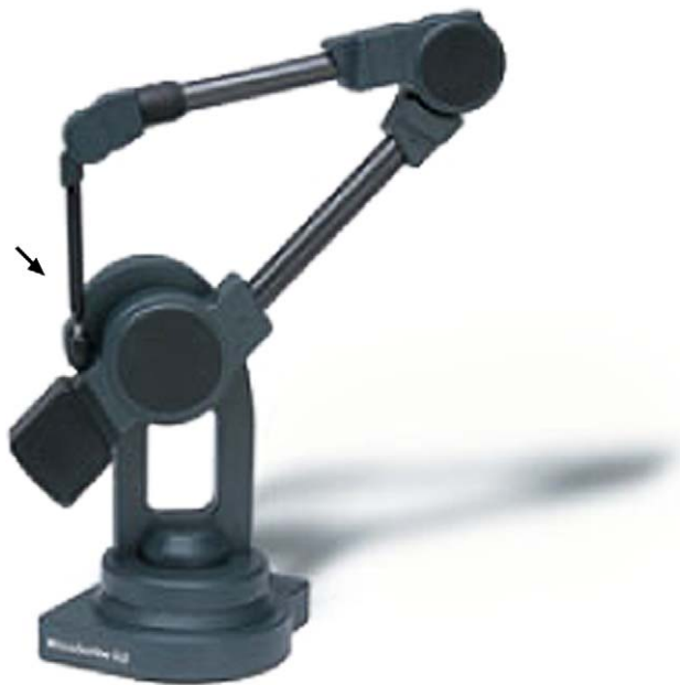
Fig. 2. A Microscribe-3DX, or digital recording device used to measure points in three-dimensional space. The arrow points to the tip of the stylus used to record start and end points for each scar.
